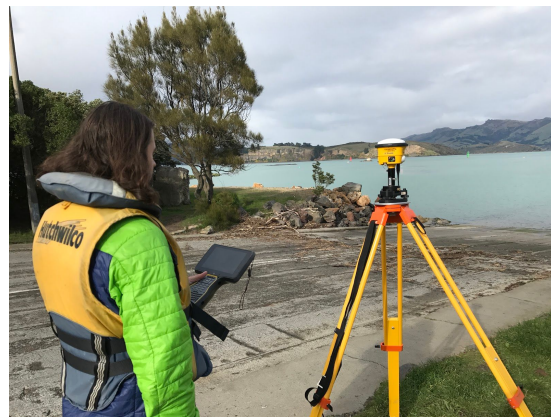
Image 3: The GNSS RTK base station used for transmitting corrections to the MPS865 receiver onboard.
