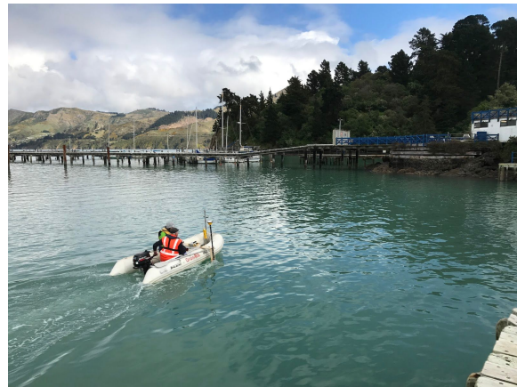
Image 1: Bathymetric survey underway using the Trimble MPS865 GNSS receiver, Siteworks field software, and Ohmex Sonarmite echosounder.
